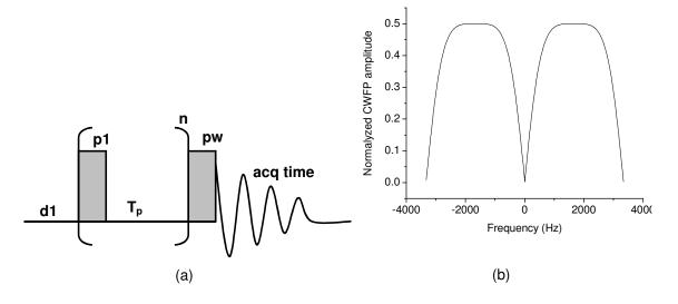
Figure 1. (a) CWFP pulse sequence; (b) excitation profile in absolute values for CWFP sequence for  $\alpha = \pi/2$  pulses and T<sub>p</sub>= 0.3ms.
