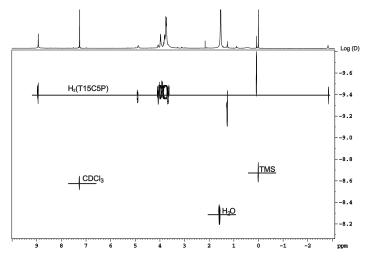
**Figure 2.** DOSY NMR spectra of H<sub>2</sub>(T15C5P), obtained using the BPPLED pulse sequence. The gradient strength of 1.6 ms duration was incremented in 32 steps, with diffusion time  $\Delta$  of 100 ms and recovery delay  $\tau_R$  of 5 ms. The *D* (diffusion coefficient) is given in m<sup>2</sup>/s.
